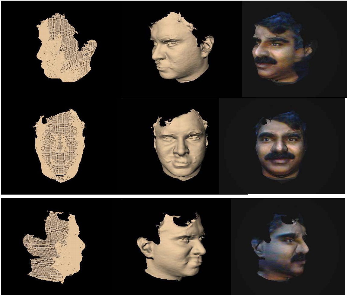
Fig. 2b. Texture Mapping using Open Inventor (face2 showing wireframe, shaded & textured in three views)
