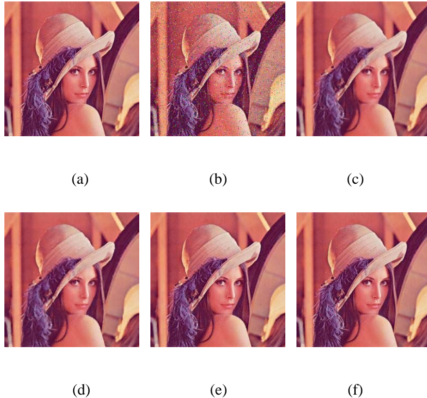
Fig. 2. Filtering results for the testing image Lena. (a) Original image. (b) Image corrupted by 4% impulsive noise. (c) Restored image using VMF. (d) Restored image using BVDF. (e) Restored image using the adaptive filter in Ref. [7]. (f) Restored image using the proposed filter
