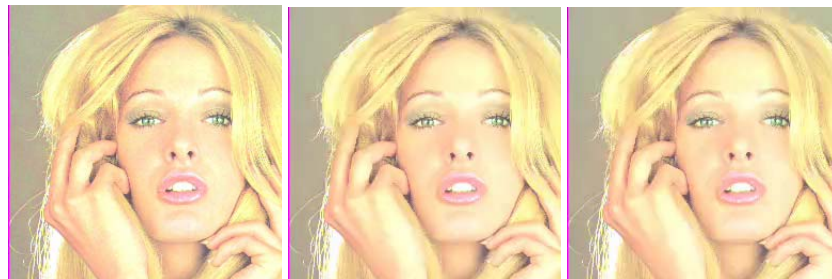
(a) Tiffany (original) (b) Encoded by H.264 I-frame encoder with QP=30 (c) Encoded by our method with QP=30
