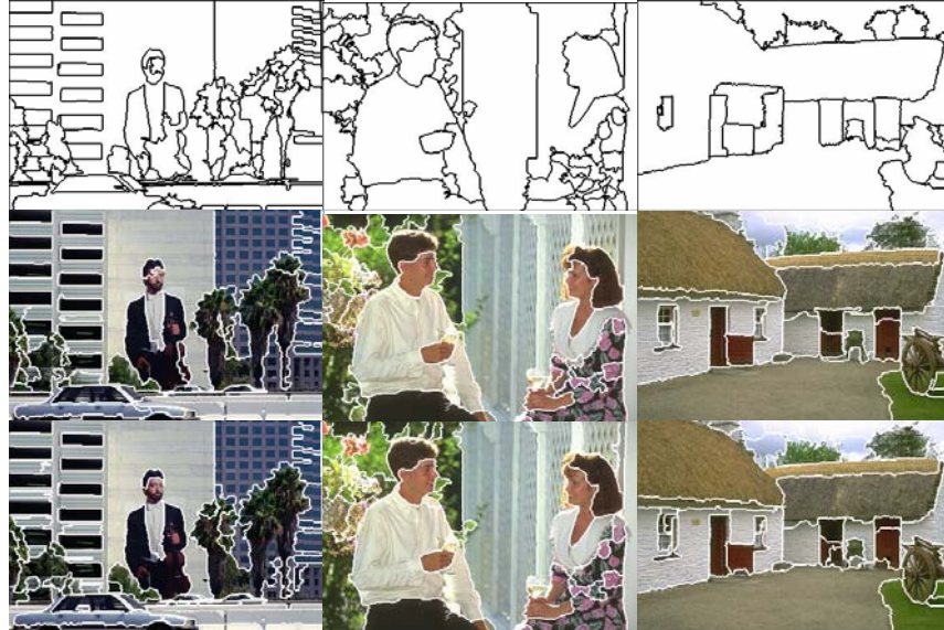
Fig.1. Comparison between mean shift and the improved clustering approach. The images in the first row are detected edges by EDISON (A mean shift clustering software). The images in the second row correspond to the improved approach with (h_s, k_h, \alpha_0, N_m) = (5, 2, 0.4, 100) . The parameters for the images in the third row are (h_s, k_h, \alpha_0, N_m) = (7, 2, 0.4, 100) .
