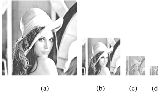
Fig. 2. Low pass components of Fig. 1 at wavelet decomposition levels (a) 1, (b) 2, (c) 3, and (d) 4 using 'Daubechies' type 4 wavelet.
