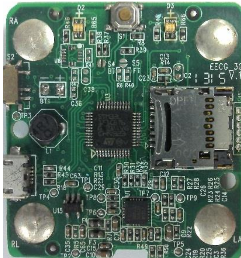
Fig. 5. The PCB board of the ECG acquisition modules
